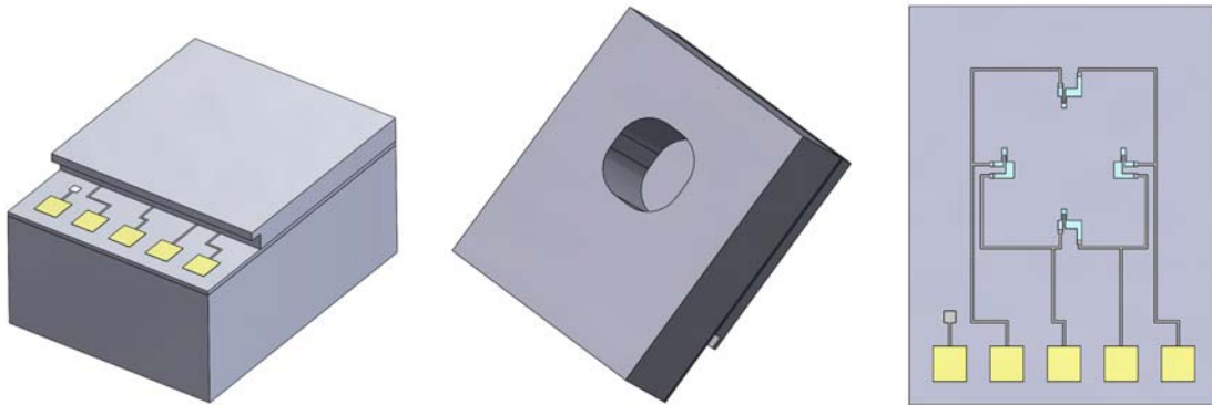
Figure 2 DRIE Hole Fabricated at NIST Nanofab
